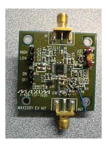
Objective: To develop and measure an external switch for maximizing power-added efficiency (PAE) with this Japanese dual-path cellular-band PA.
